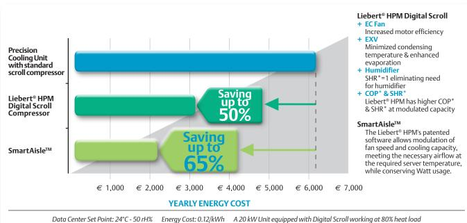
Annual savings achieved by the Liebert® HPM, complete with the most advanced technologies in the market (Digital Scroll Compressor, Electronic Expansion Valve, EC Fan) as standalone and integrated with cold aisle containment, compared to Precision Cooling units fitted with standard scroll.
